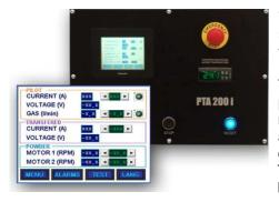
The **control panel** is in a graphic PLC with tactile screen, with functions of **programming and control of the welding parameters.**
